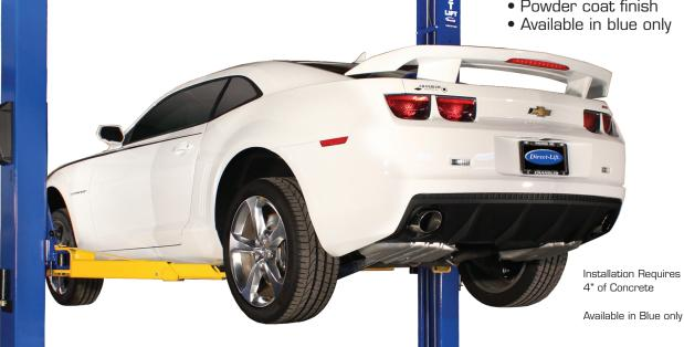
**ASYMMETRIC ARM DESIGN WITH SYMMETRIC** POST FOR EASE OF VEHICLE **ENTRY AND EXIT**
