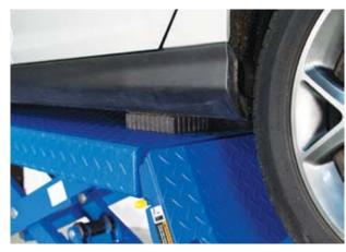
Composite polymer rubber adapter pads are placed on platforms for vehicle spotting.
