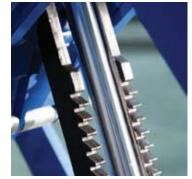
24 lock positions feature a negative rake tooth design. Locks ratchet over each other then interlock when lift is lowered to locks.
