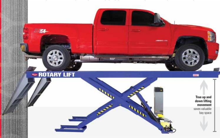
VERSATILE SCISSOR LIFT SERVICES CARS TO LIGHT COMMERCIAL TRUCKS - UP TO A 198" WHEELBASE!
