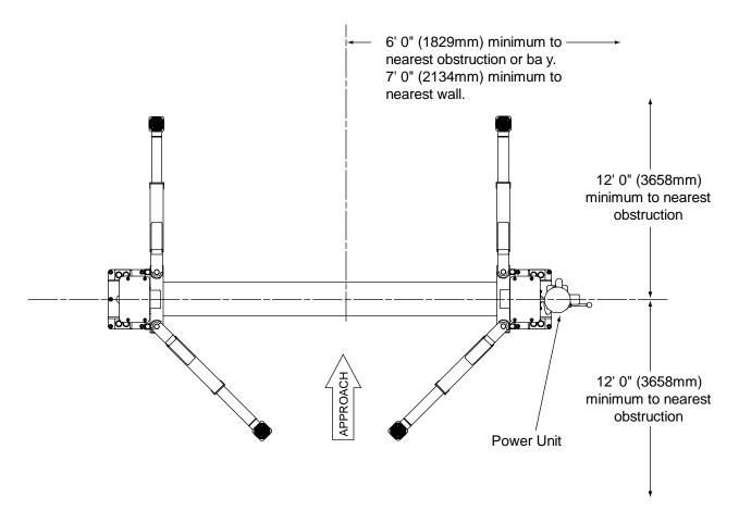
NOTE: Lift can be installed so that the power unit column can be located on either side. However, to save operation steps it is recommended that it is placed on passenger side of lift.
