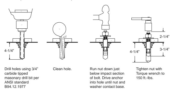
**STEP 8:** Using a level, check column for side-to-side plumb and front-to-back plumb. If needed, use horseshoe shims provided by placing shims underneath the base plate and around the anchor bolt. This will prevent bending the column bottom plates (Shim thickness should not exceed 1/2"). Tighten 3/4" anchor bolts to **150 ft-lbs.** of torque.
