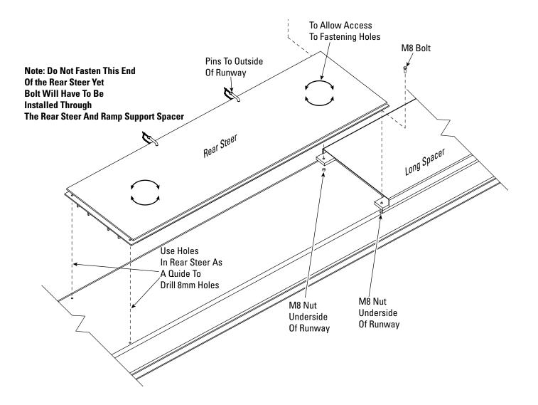
14. Slide tabs of Ramp Support Spacer under the rear of the Rear Steer. Align bolt holes and insert bolts.
